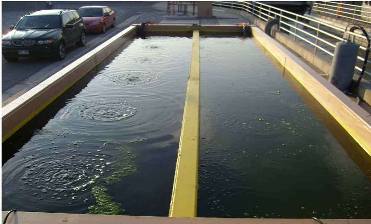
Figure 27: Side by side PG and Control tanks viewed from effluent end. Left Side: PG Tank; Right Side: Control Tank
