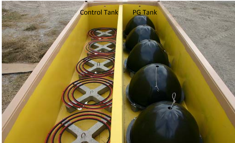
Figure 2: Overview of the dual chamber reactor tank. The Control tank with 6 bubble tube sets is on the left and the PG tank with 6 Poo-Gloos is on the right. (Nearest ones are out of the picture.) The dome structures are about 2.5' (0.762 m) high. Total tank depth is 3' (0.914 m), length is 22' (6.7 m), and overall width is 8' (2.44 m).
